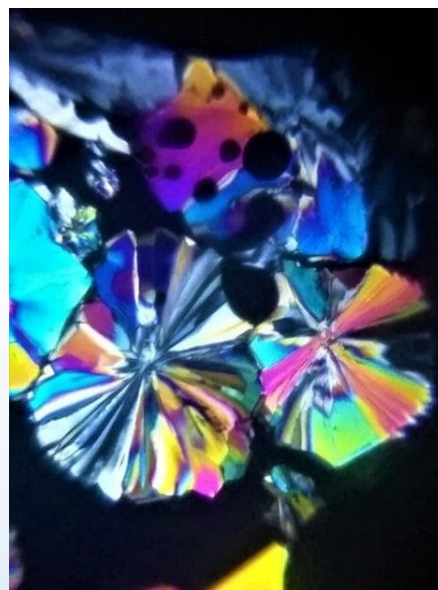
Recrystallized citric acid as seen under the microscope.
